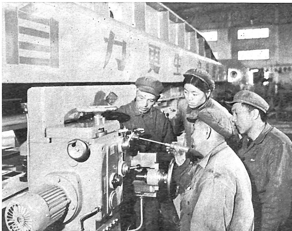
Workers assemble a large edge planer they have modified.
